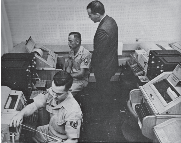
Figure 1.12 Photograph of the one-time pad machines (black) in use by the U.S. Signal Corps to support the Washington–Moscow hotline. The white machines were used to print and read plaintext messages. Photograph courtesy of the United States National Archives.
